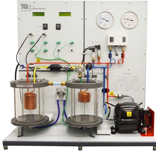
Figure 1: Refrigeration cycle board by Tecquipment
