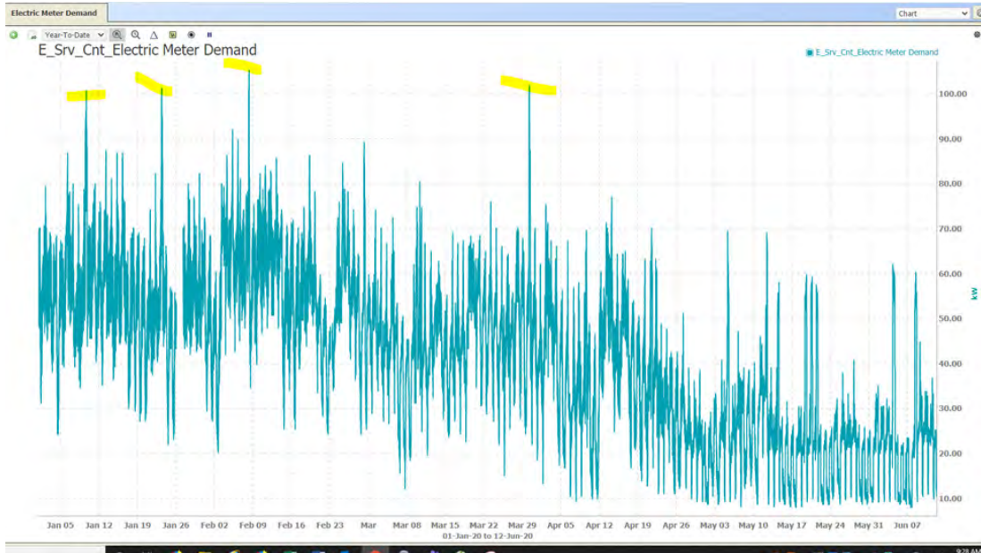
Figure 23: Eastern Service Center Energy Use Profile
